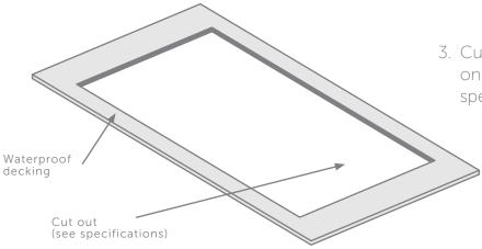
3. Cut out decking top to fit on top of bath rim, see bath specification for dimensions.
