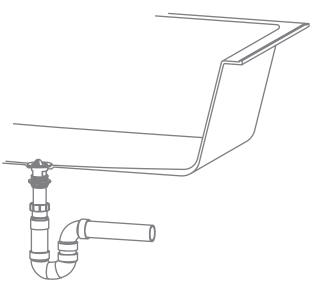
5. Install the bath waste and ensure it is connected to the PVC pipe using a flexible pipe before the bathtub is lowered into the prepared hole.
