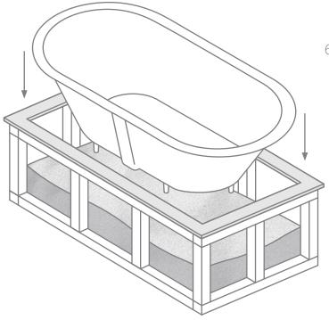
6. Drop the bathtub into the prepared hole filled with river sand, and press down until the bathtub is embedded and secured within the sand.
